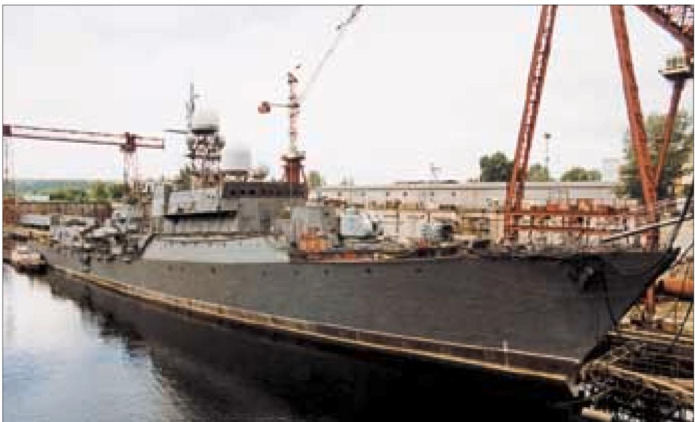
ten watertight compartments. The superstructure modules are made from aluminum-magnesium alloy which is resistant to seawater. In the event two adjacent compartments are flooded, the ship remains afloat, keeps going and continues to perform its mission.
