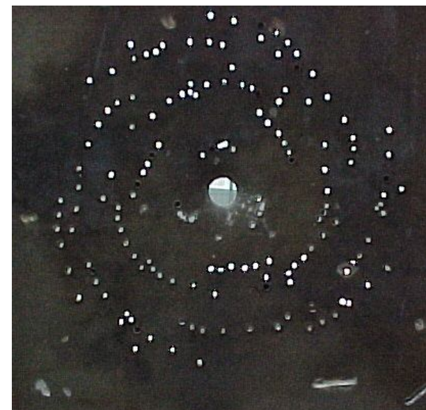
Payload-Footprint on 1 x 1 m Al-Plate after Ejection of the 162 SP (4 ms after ignition )
