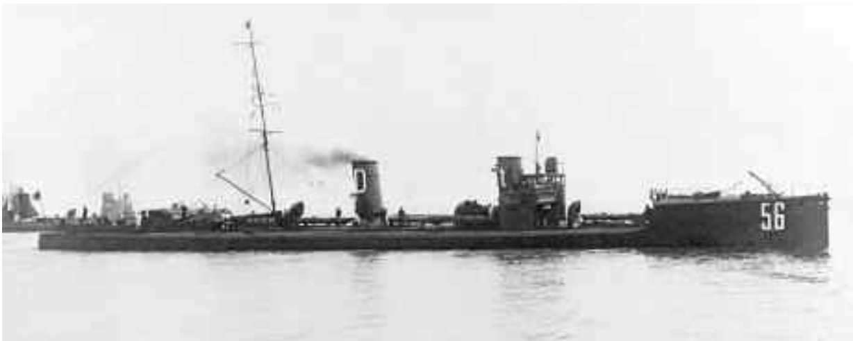
SMS V156 (1908), a typical German destroyer of the era (officially designated 'large torpedo boat'), armed with two 8.8cm guns and three single 45cm torpedo tubes. The well forward of the bridge would be a characteristic feature of German destroyers until the latter years of the First World War. V156 was one of the last German destroyers to be powered with reciprocating engines, but remained in service (latterly under the designation T156 ) until 1945. (US Naval History and Heritage Command, NH 65793)
