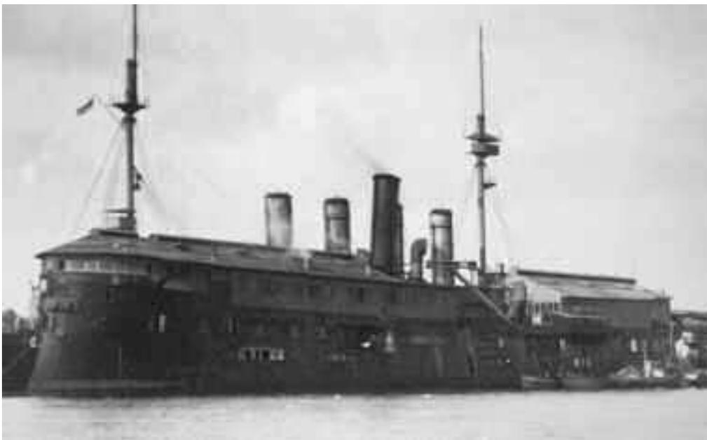
*Fisgard II* (ex-Hercules) in 1920, showing her extensive housing-in, opening up of the hull to provide interior illumination and heavy crane amidships. Her diesel generator was the main source of power for the establishment.
