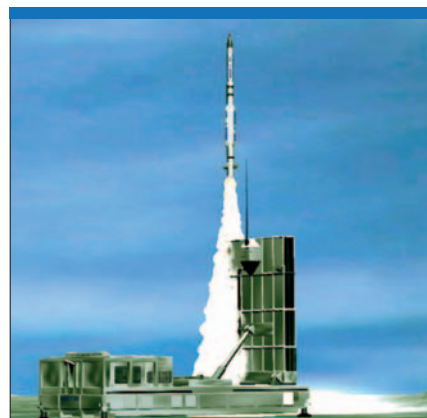
As MBDA has done with the Mica, BGT and Eads-LFK developed a VL launch system using the air-to-air Iris-T, which was unveiled at the ILA 2002 exhibition. (BGT)
