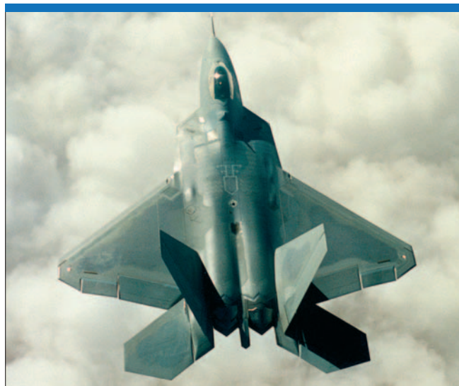
The Lockheed Martin F/A-22 Raptor combines low observability, thrust vectoring and outstanding performance. Deliveries have now begun, initially to replace the US Air Force Boeing F-15C. (Lockheed Martin)
