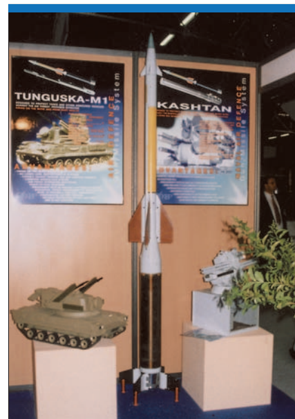
The replacement for the ZSU-23-4 Shilka is the KBP/Ulyanovsk Tunguska-M1 vehicle, which carries eight of these Fakel/KBM 9M311 (SA-19) missiles and two 30 mm cannon. (Armada/RB)
