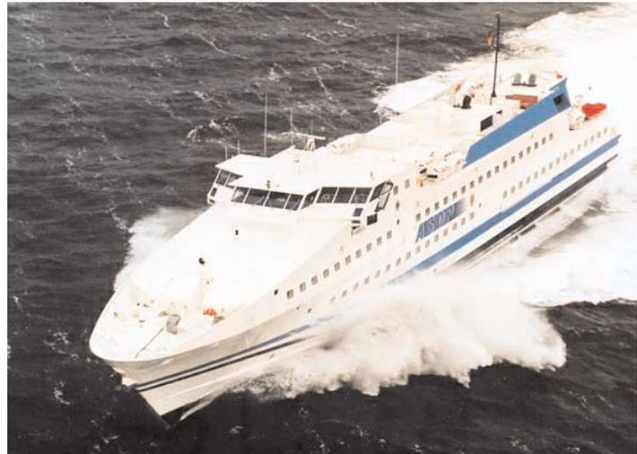
*A 43,4 m Catamaran built 1995 in Australia by Austal Ships for Diamond Ferry Company in Japan. Capacity: 331 passengers and a crew of 6. Equipped with four Kamewa 63SII she has a service speed of 42,5 knots.*
