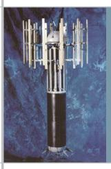
The AN/AQS-22 ALFS is the next generation integrated dipping sonar system for the MH-60R helicopter. It is the primary anti-submarine warfare sensor supporting the Navy's Helicopter Master Plan.
