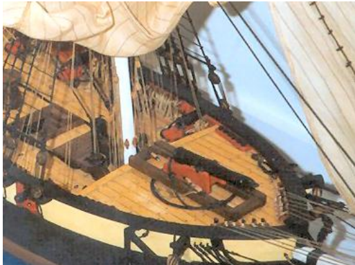
A model of the brig Oneida showing its as-designed (but never mounted) bow pivot gun. Although this is a 32 pound cannon not an 18, the Madison’s pivot gun would have looked similar. Model at the Sackets Harbor Battlefield State Historic Site, Sackets Harbor, NY; photograph by the author.
