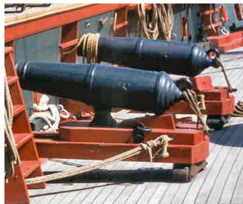
Naval carronades were usually mounted on slide carriages that were swivelled by means of a pin at the front and trucks (wheels) at the rear. Another style of carriage used a handcrew to control elevation instead of a wedge. Photograph by the author on board the brig Niagara, Erie PA, 2000.
