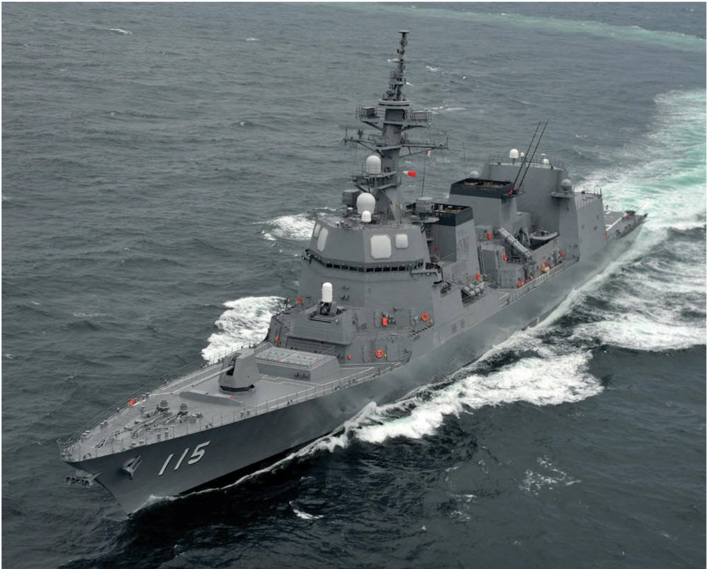
The lead Japanese Akizuki (DD-115) class destroyer pictured in April 2012, shortly after delivery. The latest in a long line of JMSDF general-purpose destroyers, the class incorporates improved local area air defence capabilities to protect specialist air-defence destroyers acting in the ballistic missile defence role. ( Japan Maritime Self Defence Force )
