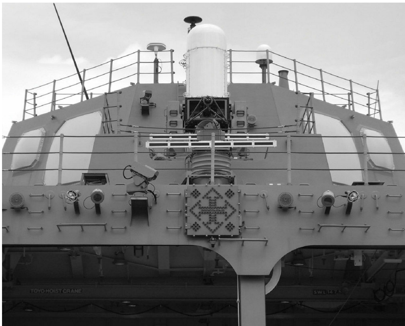
A detailed view of the aft superstructure of Teruzuki , showing the rear FCS-3A radar
