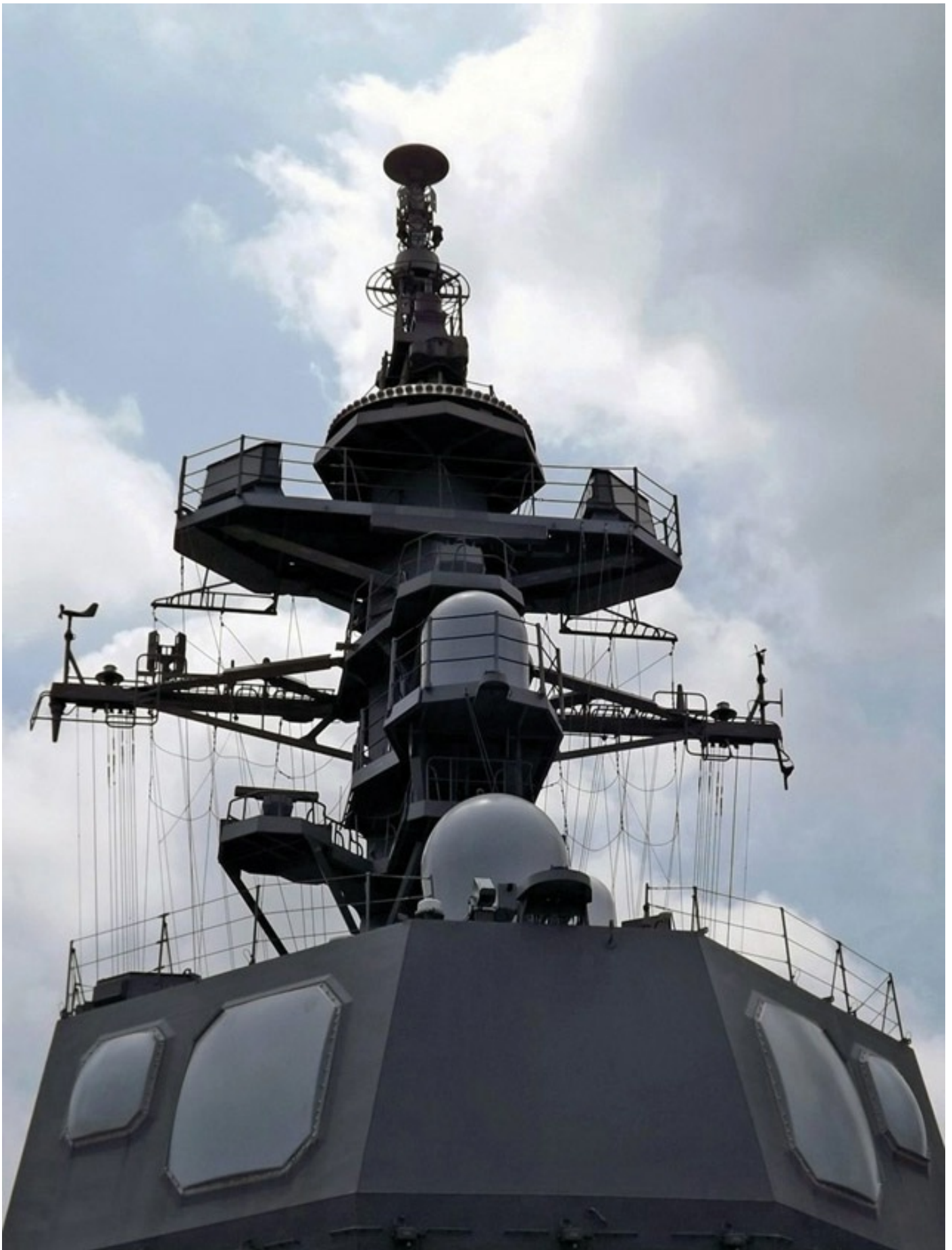
A detailed view of the forward superstructure of Teruzuki showing the paired arrays of the FCS-3A radar system. The larger arrays work in the NATO G/H bands to search for and track potential targets; the smaller arrays undertake fire control functions and operate in the higher definition NATO I/J bands. (Tomohiko Tada)
