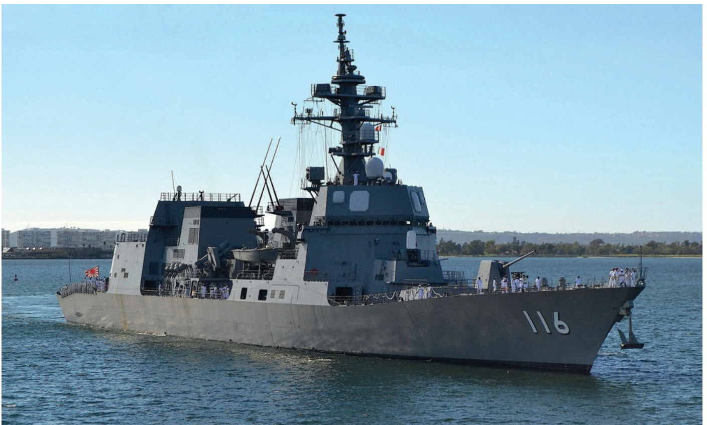
Much of the Akizuki class destroyers' principal armament is located forward of the bridge, including a long 127mm Mk 45 Mod 4 62-calibre gun and a 32-cell Mk 41 VLS
