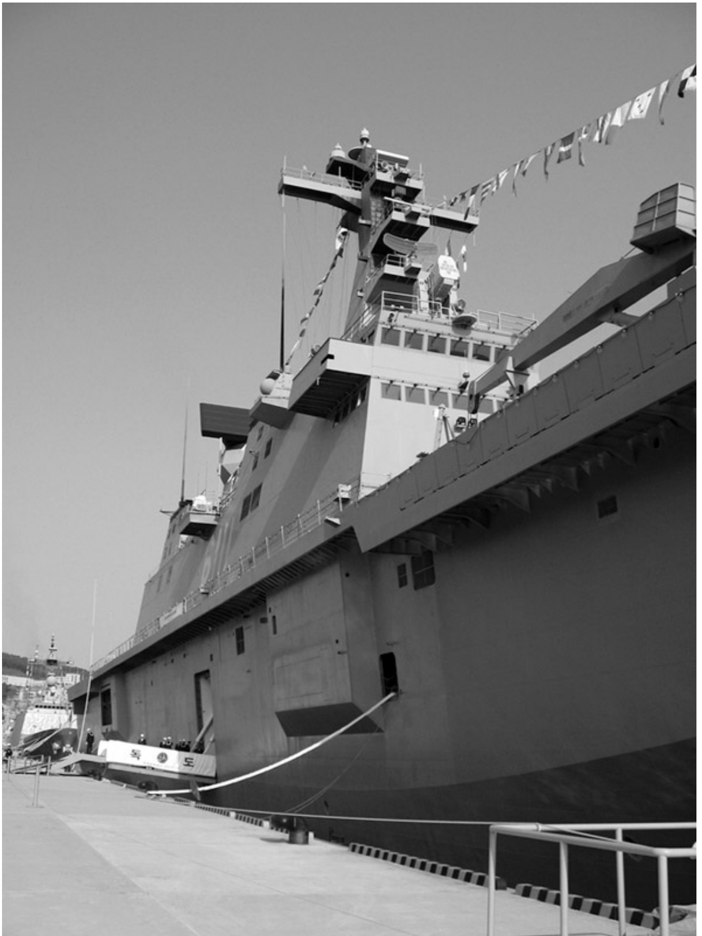
A starboard view of Dokdo , showing both the side vehicle ramp and 20-ton crane. These can be used for loading and unloading purposes when a quayside is available. (Guy Toremans)
