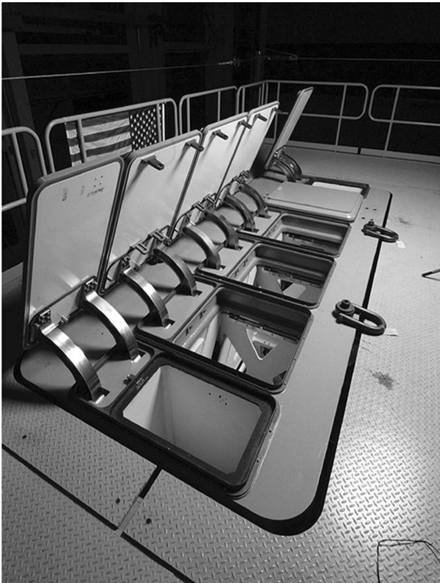
Two images showing a mock-up of a Mk 57 vertical launch system and its positioning on Zumwalt class ships. The Mk 57 system on Zumwalt comprises twenty four-cell units. Six of these are located on either side of the forecastle, with a further four on either side of the forward part of the helicopter deck. The system can handle most
